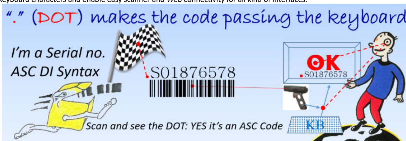
Report Fig. 10) The solution: The Flag Character "."(dot) makes the barcode data unique and passing keyboard & web interfaces
