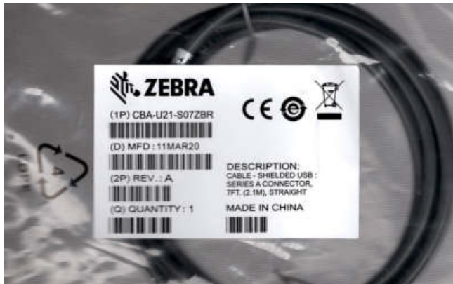
Fig. 3) Old school spare part label applied with single data elements each in one CODE 39
