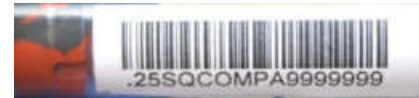
Figure 11) UIM on a test tube applied with flag character “.” → (for unique distinction with other 25S... values)
