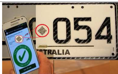
Fig. 16) DigSig verification of a QR+RFID tagged car licence plate by smart phone
