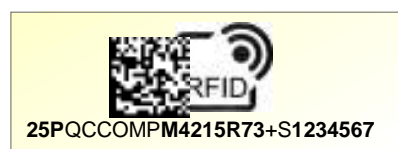
Fig. 21) Uniquely serialized product code in Data Matrix and RFID
