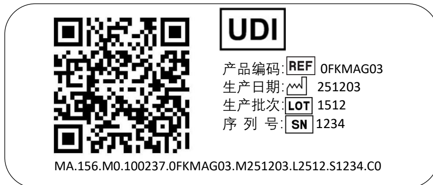
Figure 4-2 Example label using QR Code as data carrier and being applied with HRI, human translation lines in Chinese and pictograms prior to the single data values.
