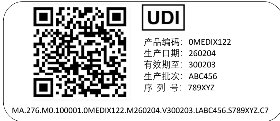
Figure 4-1 Example label with HRI, Chinese text lines for introducing the data elements of MA-UDI and QR Code as data carrier
