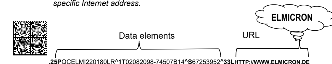
Figure 17: URL integrated in SET code using DIN 16598 KB and WEB compatible syntax.
