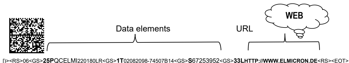
Figure 16: URL integrated in SET code using ISO/IEC 15434 syntax as link to a specific Internet address.
